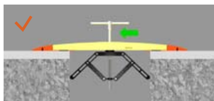
Turn the wrench clockwise until the arms of the lock key into the sides of the trench
