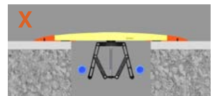
Do not attempt to open the Radlock between pipes or cables
