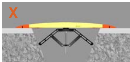
Take care to excavate a sheer trench
